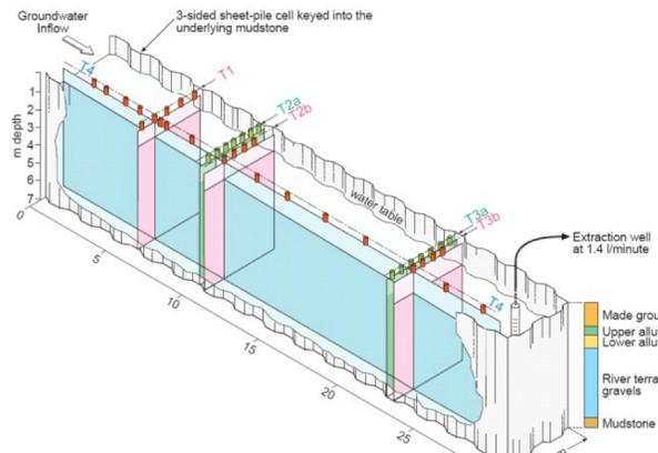
Geosyntec led the design of this sheet-piled test cell for evaluating in situ remediation of DNAPL at a former manufacturing plant
