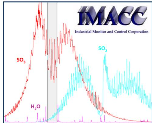
The figure at right illustrates how the intense focus of the QCL is used to resolve SO<sub>3</sub> absorption spectra with very little biasing from SO<sub>2</sub> & H<sub>2</sub>O. Detection limits are about 250 ppb for NH<sub>3</sub> and SO<sub>3</sub> in dust-free (laboratory) environments and as low as 0.5-2.0 ppm in the field, with less than one minute sample times.
