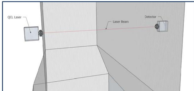
During operation, lime was injected upstream for SO<sub>3</sub> mitigation, meaning both fly ash and solid sorbent were present in the duct during testing. The analyzer ran unattended, with data sent wirelessly to a location offsite for processing and analysis.
